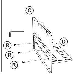
Step 3: Attach side (B) to panels (C & D) with 3 screws (R), using the included hex wrench.
