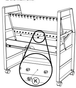
Step 9: Install the 17 plastic dividers (J) to the main unit. You have completed assembly.
