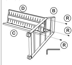
Step 4: Attach side (A) to panels (C & D) with 3 screws (R), using the included hex wrench.
