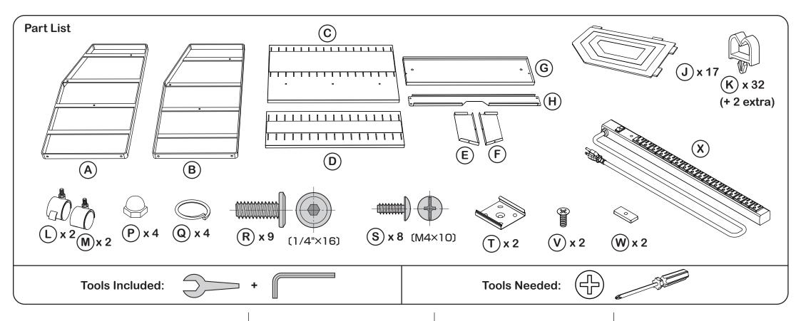
Step 1: Attach the casters (L & M) to the side frames (A & B) with the lock washer (Q) and acorn nut (P), using the included wrench.
